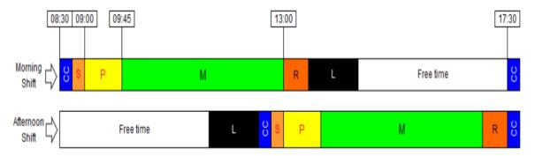
It is important to have the reset-time between shift changes. During this reset-time the control-unit is cleared, machine parameters are reset to original stage, and tools and tool holders are taken out. The machine is cleaned by the Competitor and made ready for the next shift to start their Test Project.
